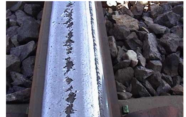
Rolling Contact Fatigue
