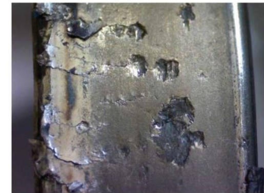
Surface after 200 000 cycles, Severe Spalling
